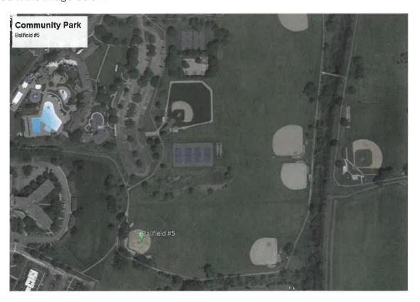
The problem with this field, essentially, is its location in the park. Surface drainage has long been an issue as the topography of that section of the park is pitched to the west (left on the above image). This results in the infield material being washed into and through the third base dugout, across the asphalt path that feeds the field, onto the adjacent main path and to the north, towards Discovery Playground. Below is an image of the area after a moderate rain:
